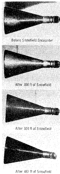
Fig. 4 Sequence of in-flight front-lighted laser photographs.
